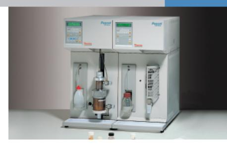
Many solid and powder materials both natural (stones, soils, minerals, etc.) and manufactured (catalysts, cement, pharmaceuticals, metal oxides, ceramics, carbons, zeolites, etc.) contain a certain void volume of empty space. This is distributed within the solid mass in the form of pores, cavities, and cracks of various shapes and sizes. The total sum of these void volumes is called porosity.
